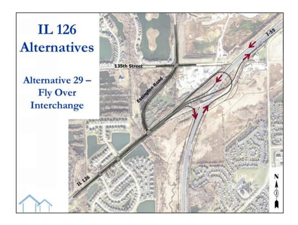
Alternative 29 proposes a flyover interchange at IL 126. \* This alternative would realign ramps to and from northbound I-55 and would provide new ramp access to and from southbound I-55.
