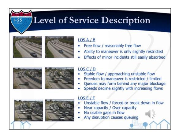
It is important to note how the level of traffic is defined. The amount of traffic on a facility, or level of service, is rated on a scale from A to F. LOS A and B indicates at or near free flow traffic. LOS C and D begin to approach unstable flows
