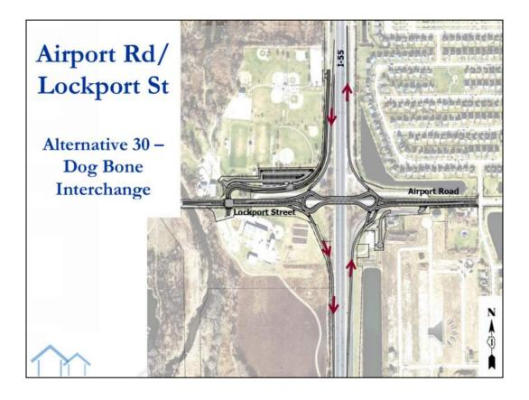
The second alternative located at Airport Road/Lockport Street is Alternative 30, the Dog Bone Interchange.\* The dogbone alternative would provide access to and from I-55 in the northbound and southbound directions, however, instead of using traffic signals for traffic control, the interchange will operate with two roundabouts.
